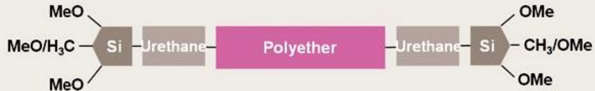
Figure 1: In currently available silane-terminated polymers, the polypropylene glycol (PPG) backbone is terminated with silane groups either directly (in SPEs) or via a urethane group (in SPURs).
