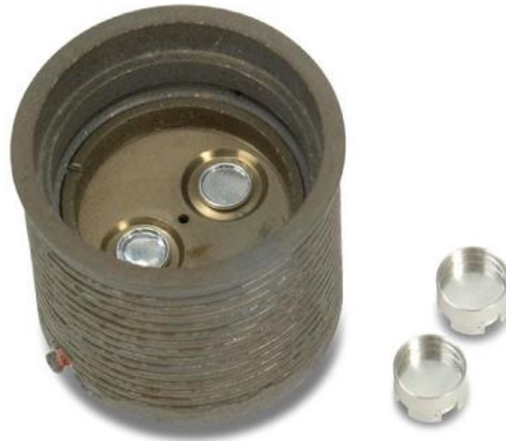
Figure 2. The double-furnace design pictured on the right allows very fast cooling and heating required for isothermal crystallization studies.
