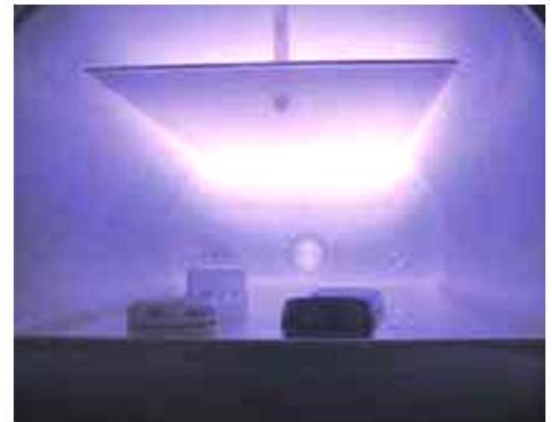
fig. 18 : oxygen plasma, low pressure
